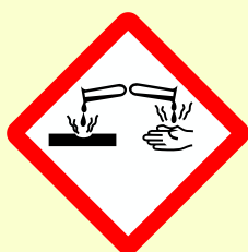
CORROSIVE ACID WARNING SIGN
